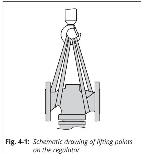
**Fig. 4-1:** Schematic drawing of lifting points on the regulator
