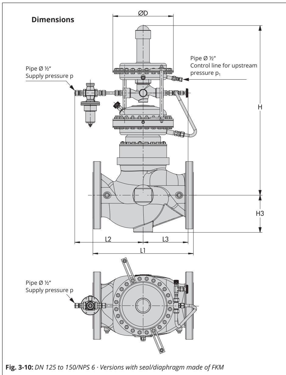
Fig. 3-10: DN 125 to 150/NPS 6 · Versions with seal/diaphragm made of FKM
