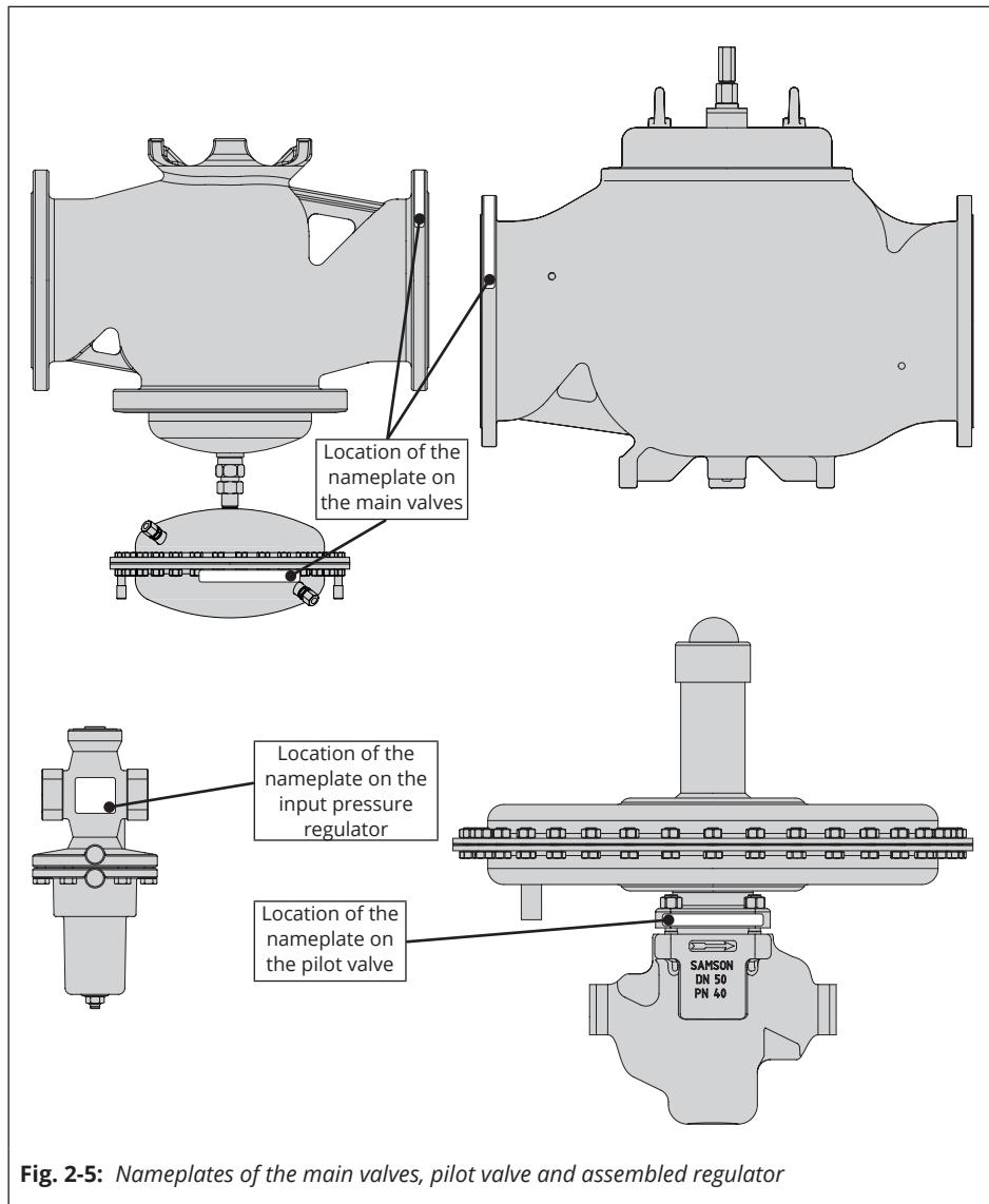
Fig. 2-5: Nameplates of the main valves, pilot valve and assembled regulator
