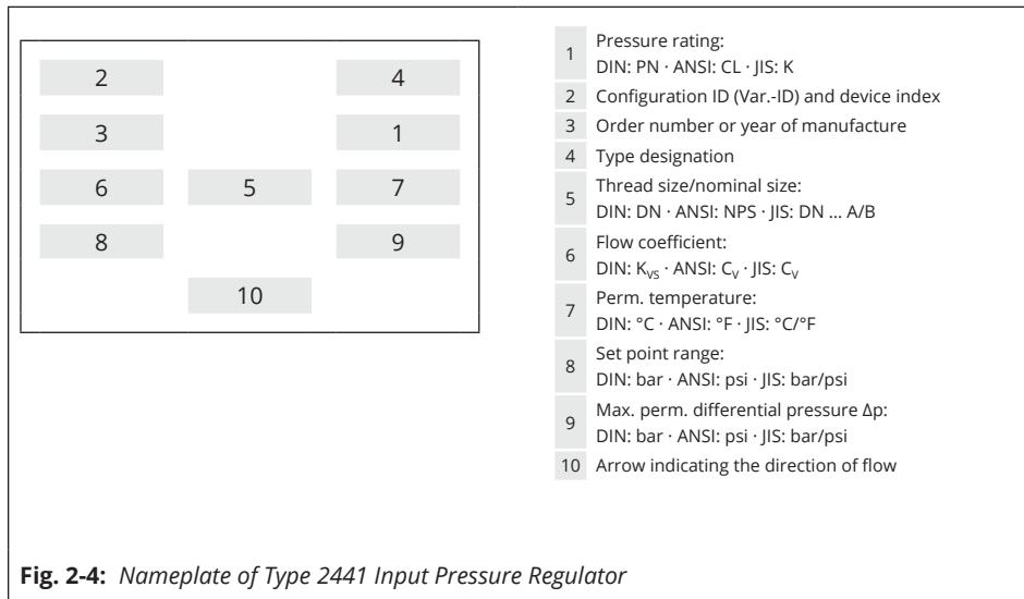
**Fig. 2-4:** Nameplate of Type 2441 Input Pressure Regulator
