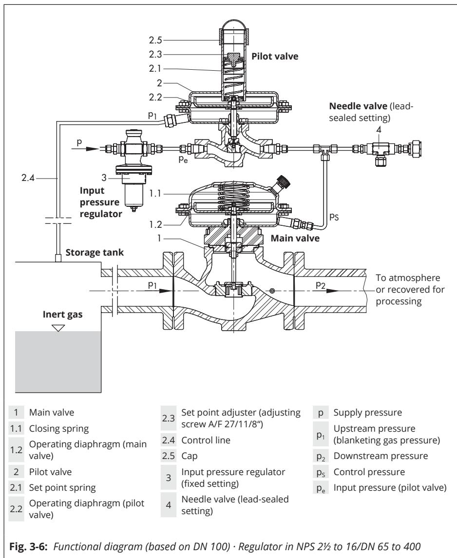
**Fig. 3-6: Functional diagram (based on DN 100) · Regulator in NPS 2½ to 16/DN 65 to 400**
