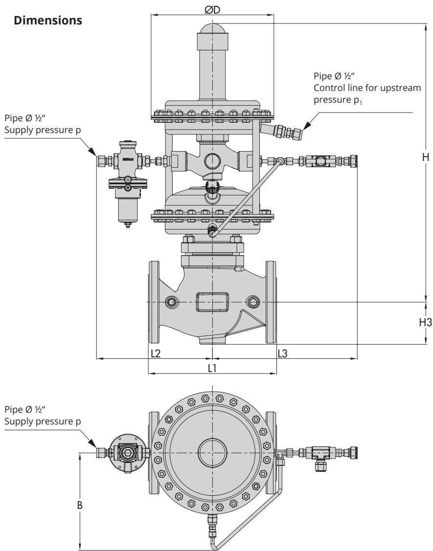
**Fig. 3-8: DN 65 to 100/NPS 2½ to 4 · Versions with seal/diaphragm made of EPDM/NBR/FKM**
