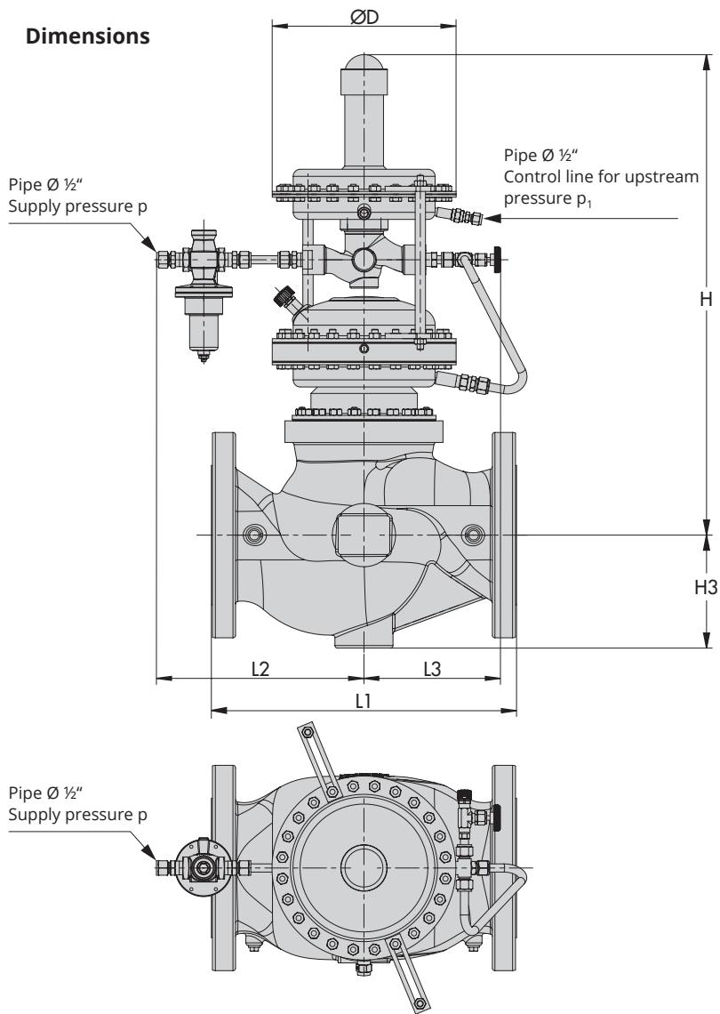
Fig. 3-9: DN 125 to 150/NPS 6 · Versions with seal/diaphragm made of EPDM/NBR
